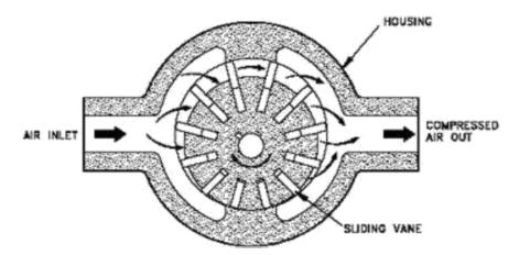
This type of compressor, looks and functions like a vane type hydraulic pump. An eccentrically mounted rotor turns in a cylindrical housing having an inlet and outlet. Vanes slide back and forth in grooves in the rotor. Air pressure or spring force keeps the tip of these vanes in contact with the housing. Air is trapped in the compartments formed by the vanes and housing and is compressed as the rotor turns.
