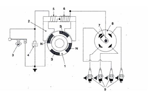
Rotating magnet; 2. Armature pole piece; 3. Cam;
