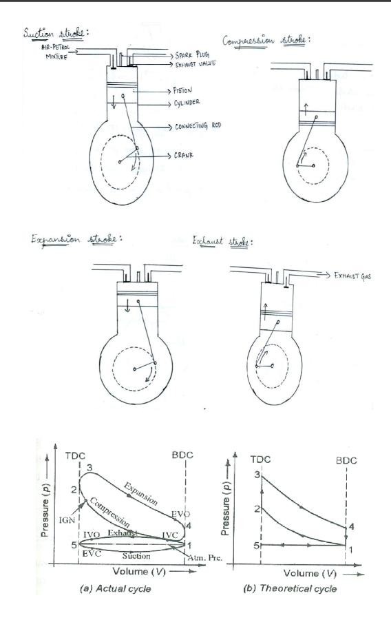
Actual cycle & Theoretical cycle for four stroke cycle S.I Engine
