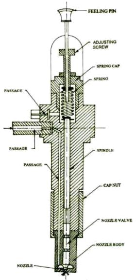
Fig. Fuel injector
