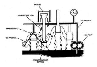
**Fig: 5 Pressure Lubrication System**
