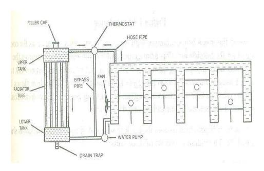
Fig: 2 Water Cooling System
