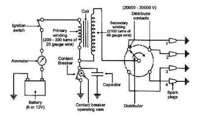
Fig: 4 Battery Ignition System
