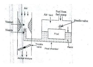
Fig:3 Simple Carburettor
